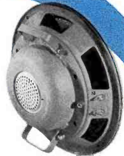
756A 10" direct radiator, power handling capacity 20 watts, response 65 to 10,000 cps.
